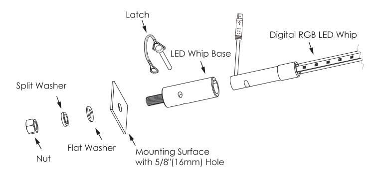
Caution! Check both sides of the mounting surface for obstruction visually before starting. If damage to other components is likely, select a different mounting location/position.
